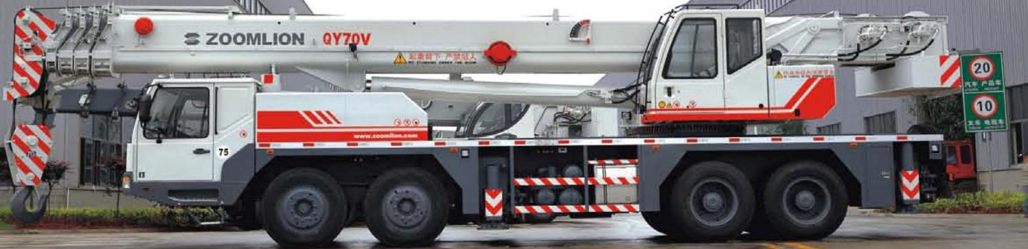
Five-section hexagonal boom, max lifting height of main boom reaches 44.2m, and its max. lifting height with 2-section jib reaches 60.2m;
